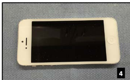
Figure 4: Post QAC wipe mobile phone was left wet for two minutes and air dried per manufactures instructions. Post wipe residue present.
